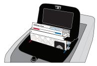
**Warning:** If the pouch does not load easily ensure that lid is opened completely.
