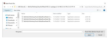
**NOTE:** The BioFire Global Fever v2.1 Panel requires three .dll files which must be installed one at a time.
