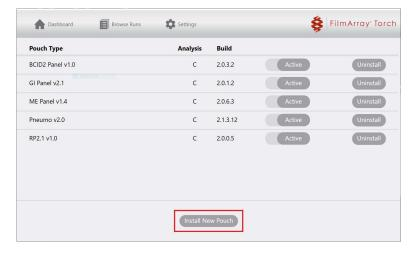
4. Select the 'Install' option associated with the desired pouch module.
